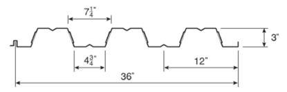
**Form deck** is used extensively in floor construction as an economical form to support concrete slabs during construction where a steel/concrete composite is not required. Finishes:
